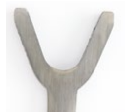
Unretouched photograph of a section cut from a flame- hardened McKissick sheave (etched 2-1/2 minutes)
