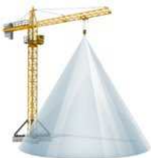
Unobstructed view of load and surrounding area below
